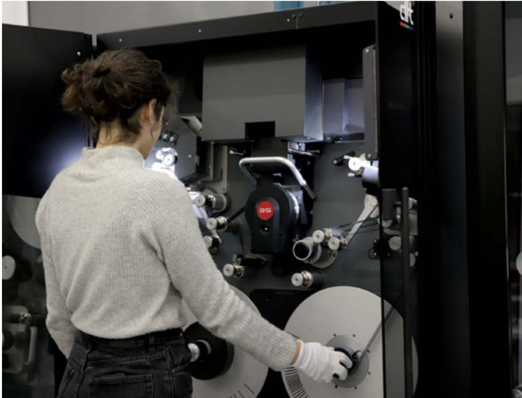
High-performance system for film digitization; photographer: Fidel Gonzalez Armatta, Federal Archives
