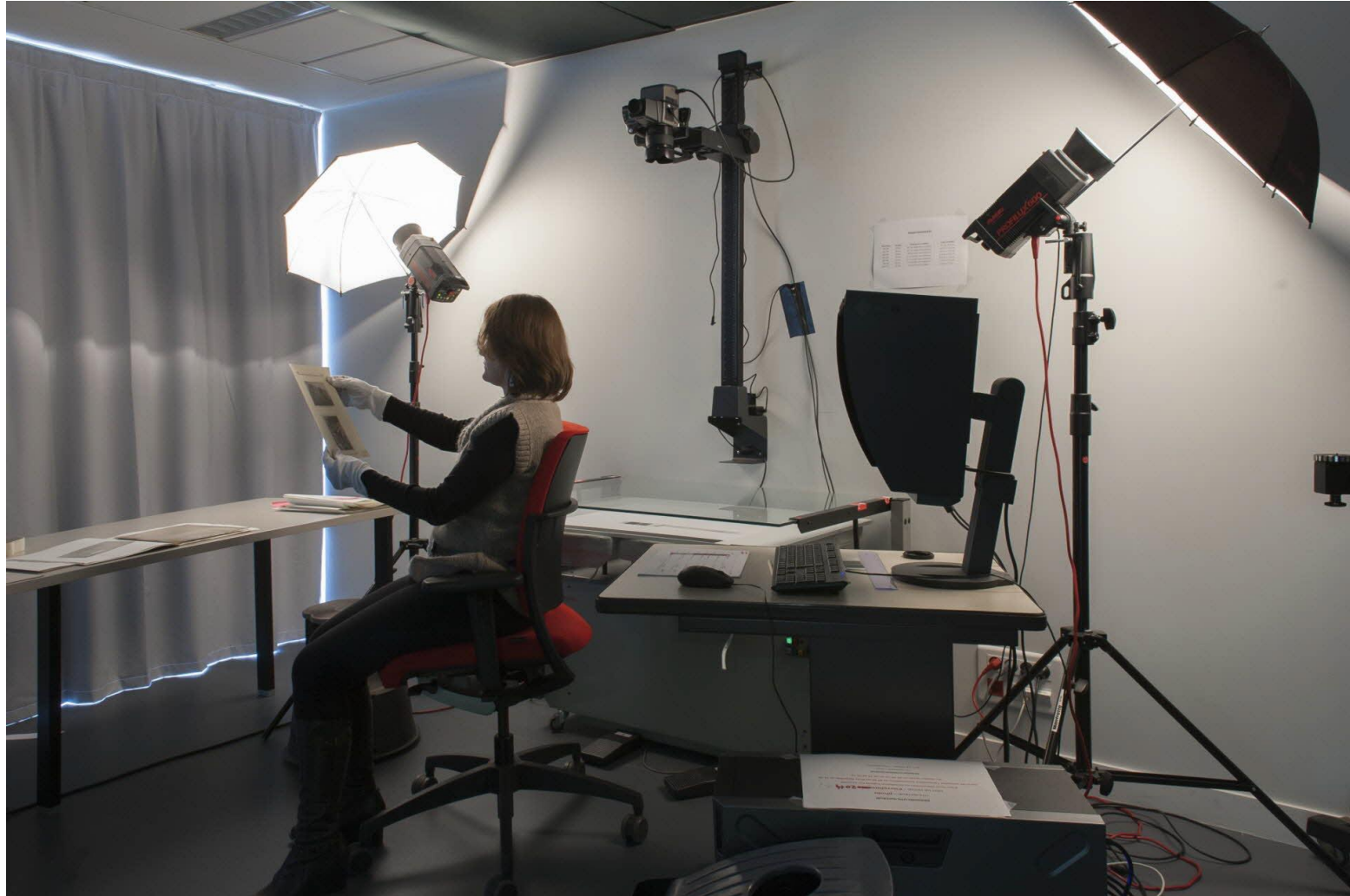
digitization workshop for A1 item or books with glass and book holder
