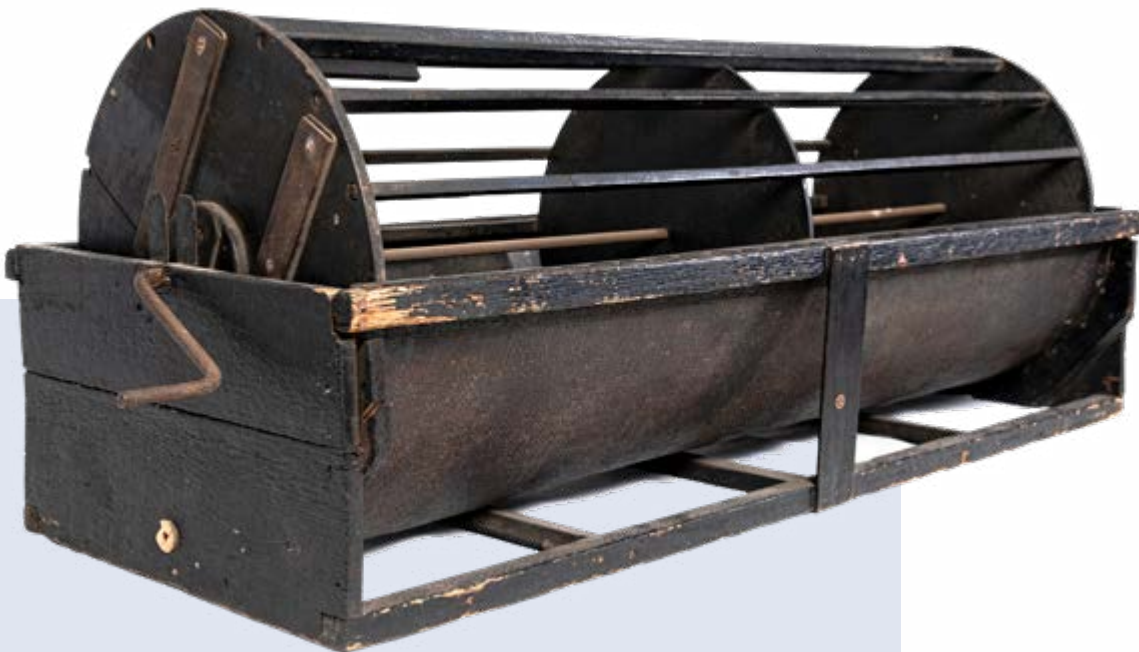
Development Drum (Measurements in cm: 135 x 34 x 35 / L x W x H / Material: softwood frame, drum made of hardwood, metal bars and rods)
